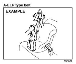
3) Allow the extra webbing to retract, and pull the webbing toward the retractor to take up any slack. Make sure that the lap portion of the belt is tight around the child restraint system and the shoulder portion of the belt is positioned so that it cannot interfere with the child's head or neck.
